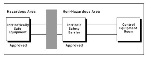
Most applications require a signal to be sent out of or into the hazardous area. The equipment mounted in the hazardous area must first be approved for use in an intrinsically safe system. The barriers designed to protect the system must be mounted outside of the hazardous area in an area designated as Non-hazardous or Safe in which the hazard is not and will not be present.
