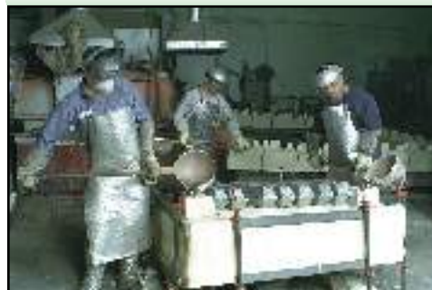
Processing aluminum castings using a Sand Mold.
