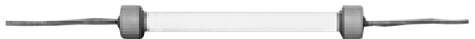
Type L1 Straight-Out Leads 10" flexible lead wire externally spliced standard. If longer leads are required, specify.
