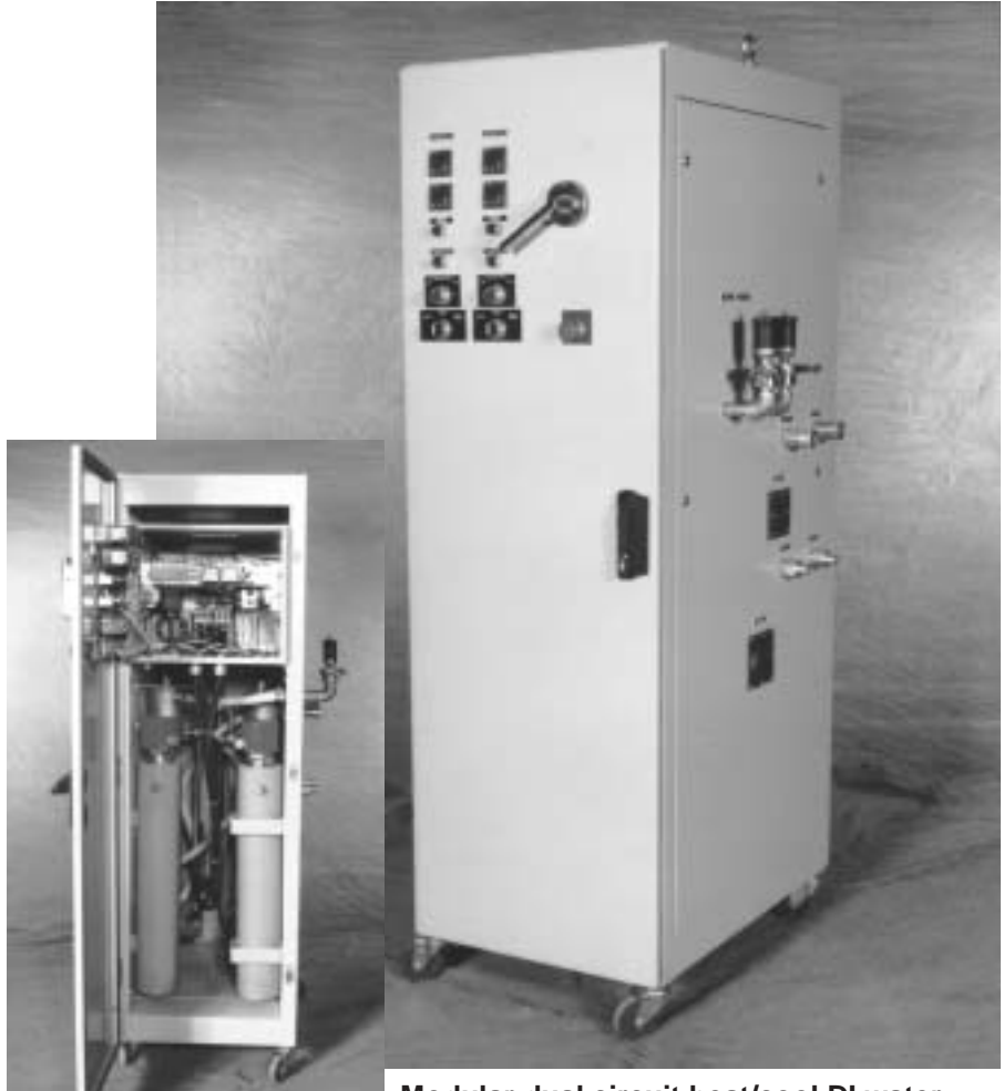
Modular dual circuit heat/cool DI water system fully enclosed in cabinet with castor wheels.
