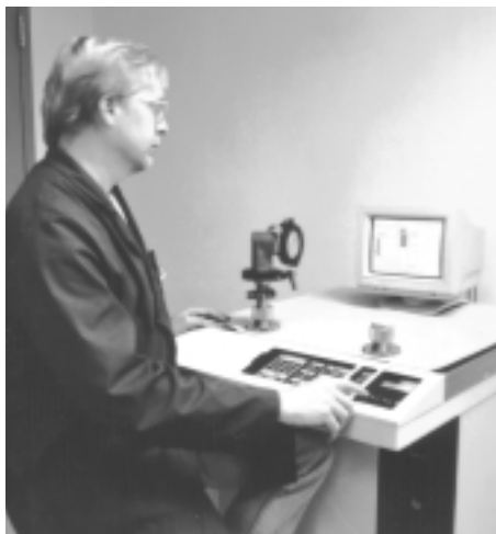
A lab service technician performs a helium leak test to verify fitting integrity.
