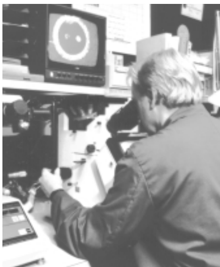
A lab service technician uses a metallurgical microscope to examine the microstructure of the metallic components in our mineral insulated metal sheathed cable, XACTPAK®.
