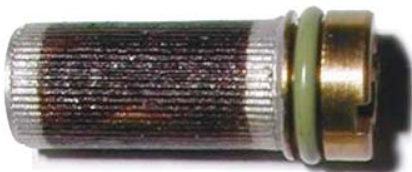
Last chance filters on moog valve before Kleentek.
