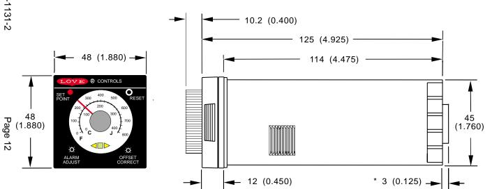
Panel cutout for all models is 45mm x 45mm (1.775in x 1.775in). Allow for 13mm (0.5in) clearance at the rear.
