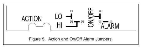
Select the action by placing the ACTION jumper to either LO (direct acting) or HI (reverse acting). The ON/OFF ALARM jumper determines whether the output will reset after the temperature has moved to the other side of the set point. If ON/OFF is selected then the output will automatically reset. If ALARM is selected then the RESET button on the front of the control must be pushed before the output will reset.
