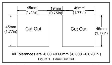
From the front of the panel, slide the housing through the cut out. The housing gasket should be against the housing flange before installing. From the rear of the panel slide the mounting collar over the housing. Hold the housing with one hand and using the other hand, push the collar evenly against the panel until the spring loops are slightly compressed. The ratchets will hold the mounting collar and housing in place.
