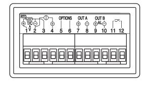
the screw clockwise to tighten. Maximum torque is 0.424 N·m(3.75 in. lb.). Do not overtighten. The wire should be held snugly in place.
