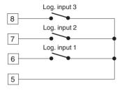
Fig. 7 - LOGIC INPUT WIRING
