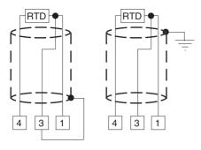
Fig. 5 RTD INPUT WIRING
