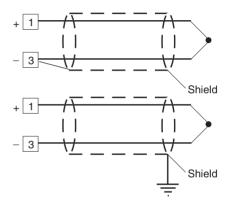
Fig. 4 THERMOCOUPLE INPUT WIRING
