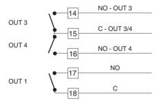
Fig. 9 RELAY OUTPUTS WIRING
