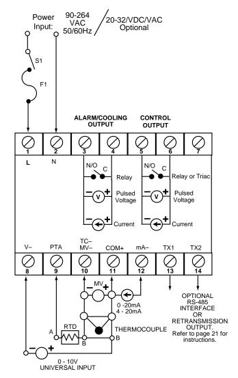
**Figure 4.3 Rear Terminal Connections**
