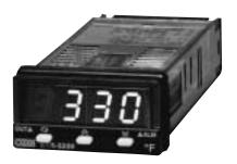
DISPLAY AFTER INPUT SHIFT. ADJUST SET POINT TO 330
