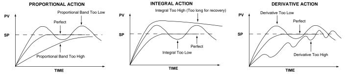
Fig. 5.2 Effects of PID Adjustment of Process Response
