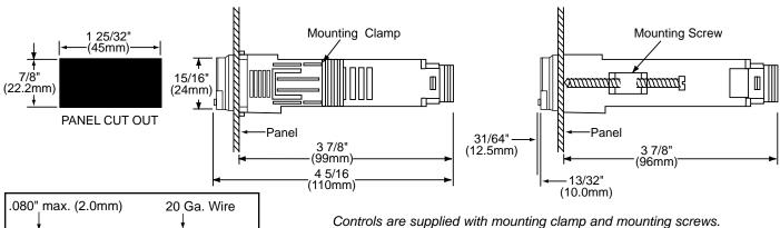
Controls are supplied with mounting clamp and mounting screws.
