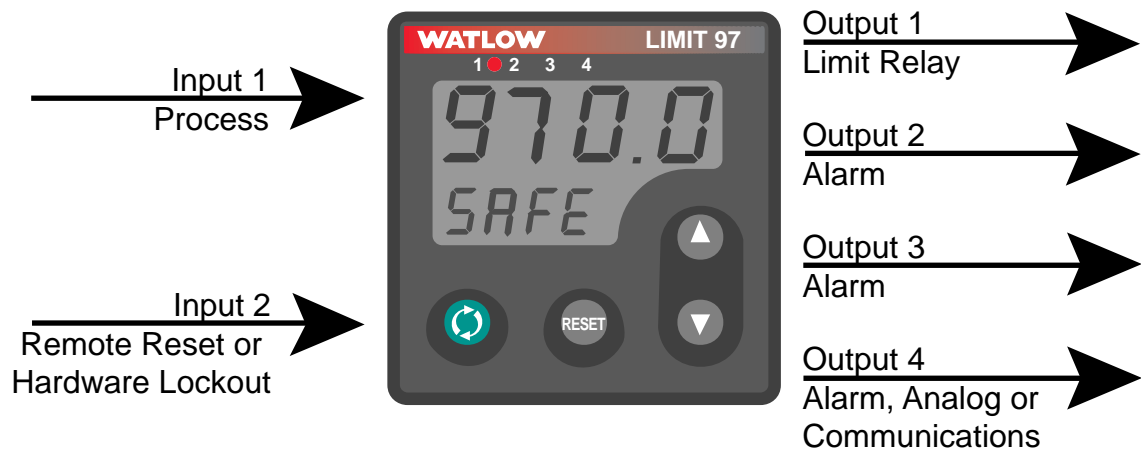
Figure 1.1 — Series 97 inputs and outputs.
